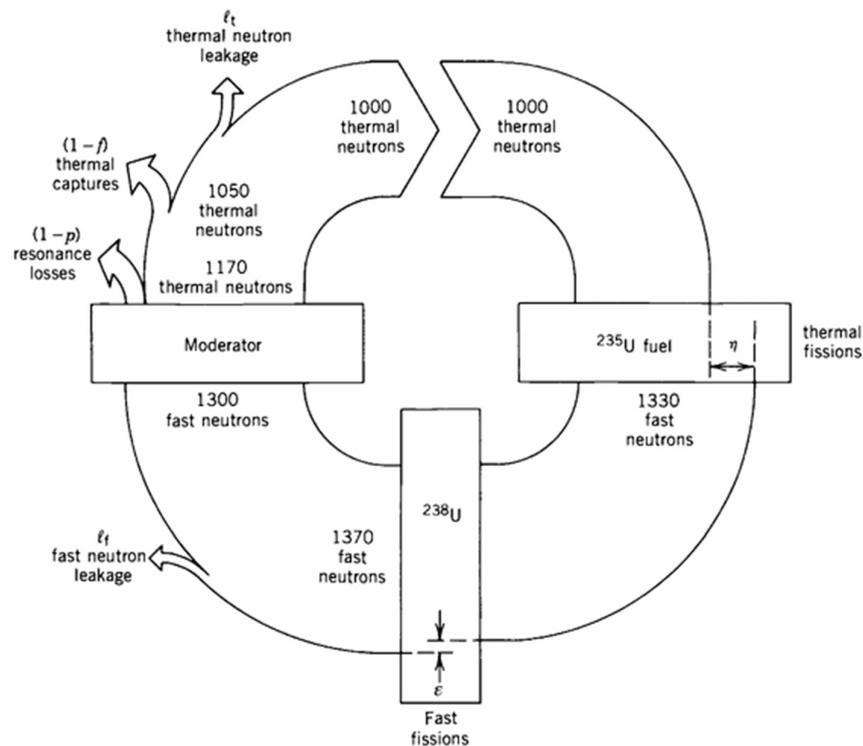
Schematic representation of processes occurring during a single generation of neutrons. The cycle has been drawn for a reproduction factor  $k$  of exactly 1.000.
